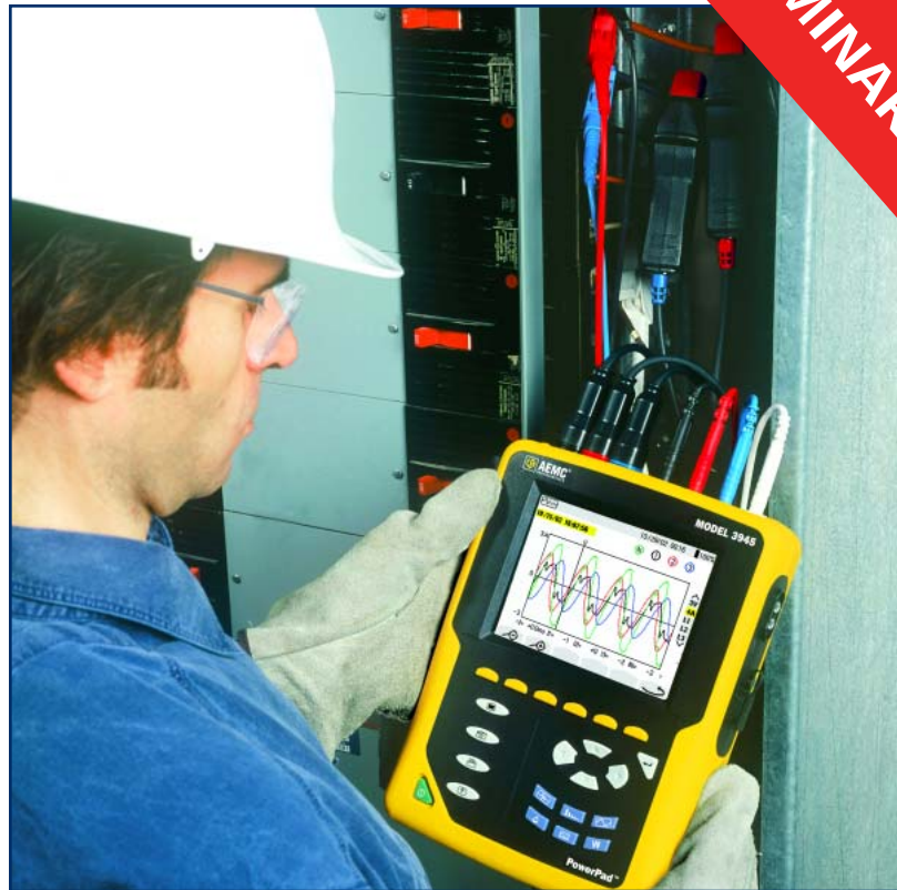
Waveform analysis of phase and neutral currents
