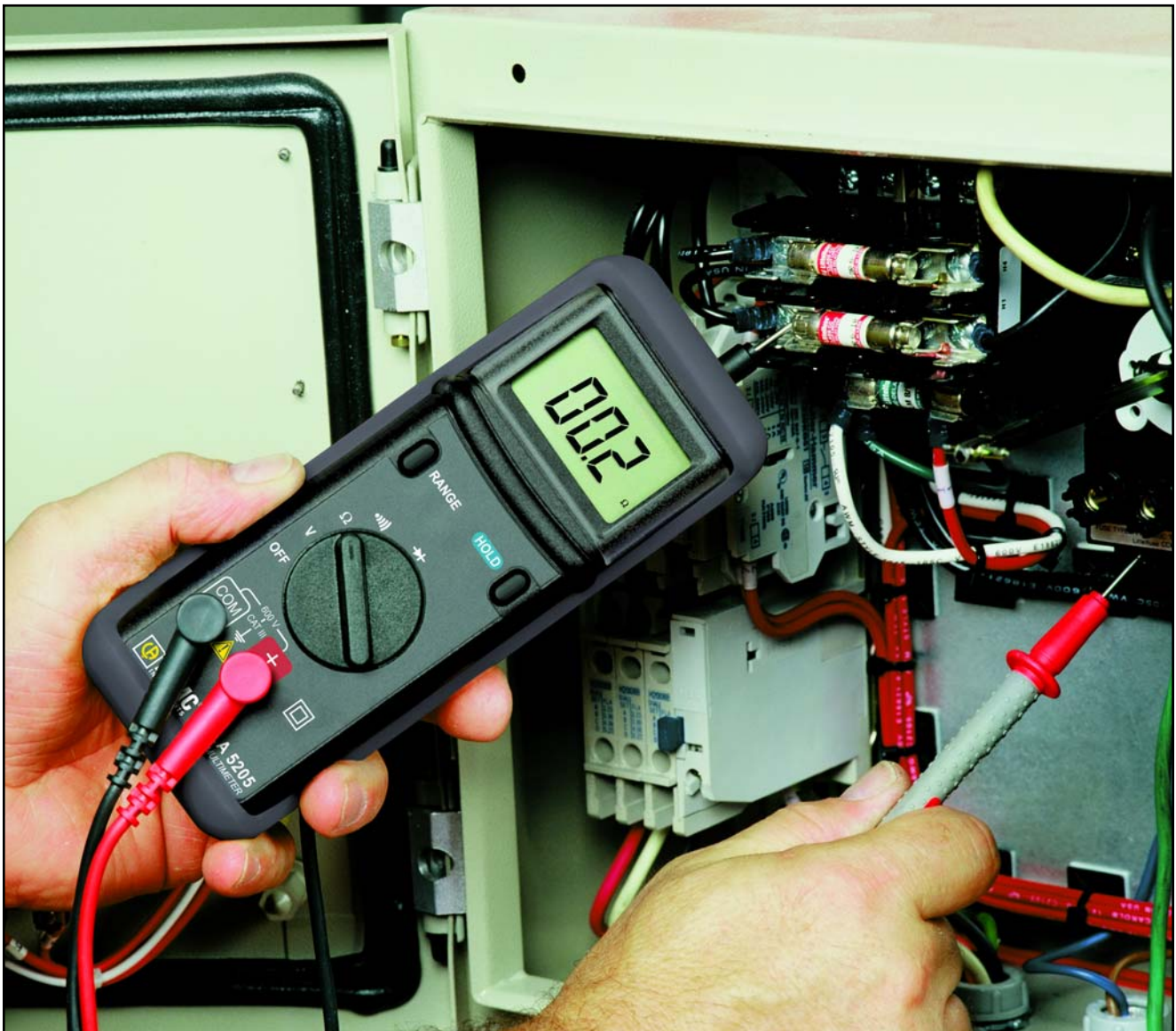
Model CA5205 measuring resistance in a relay cabinet.
