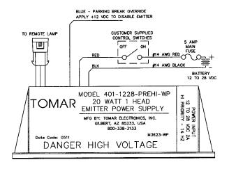
The Model 401-1228-PREHI Emitter Power Supply is designed for mounting on a sturdy flat surface protected from rain, spills, excessive heat, and physical damage. It may be installed in the trunk of a car, the saddlebag of a motorcycle, or other similar protected location. This device may also be installed in the engine compartment of a vehicle as long as it is mounted to a sturdy, flat surface, as far away from the engine as possible.
