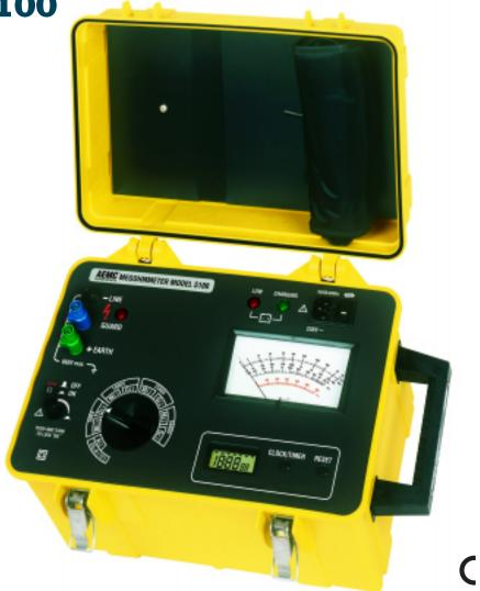
True Megohmmeter® Model 5100 is a portable, multiple-range, high sensitivity megohmmeter capable of measuring a wide range of insulation resistances from  $10 \mathrm{k}\Omega$  up to  $3000 \mathrm{G}\Omega$ . The Model 5100 has four test voltages: 500V, 1000V, 2500V and 5000V. Each test voltage setting has two overlapping resistance ranges of 30 to  $30,000 \mathrm{M}\Omega$  and 3 to  $3,000,000 \mathrm{M}\Omega$  ( $3T\Omega$ ).
