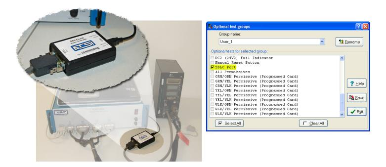
The SLNK-3000 connects directly to Port 1 of the MMU with a supplied 15 pin D-sub cable, and connects to the computer that is running the PCMT-2600 software via a USB connection.
