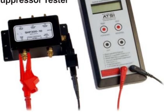
The ATSI SST 450 Suppressor Tester is designed to quickly and easily test all commonly used transient voltage suppressors: metal-oxide varistors (MOVs), gas-discharge tubes (GDTs), silicon avalanche diodes (SADs), thyristor surge protective devices (TSPDs), and hybrid devices.
