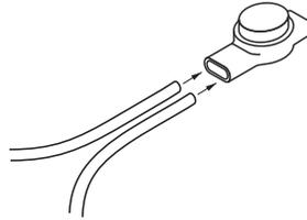
To make the splice, insert the unstripped ends into the connector as far as they will go. Then use pliers to compress the button down approximately flush with the connector body.
